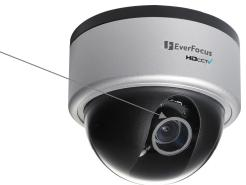
Push the interior cover toward the base, until it completely covers the whole red gasket and is lined up parallel with camera base. (The cover must be aligned with the camera base or it cannot be closed. Then turn the outer cover ring clockwise to secure it tightly to the camera base.
